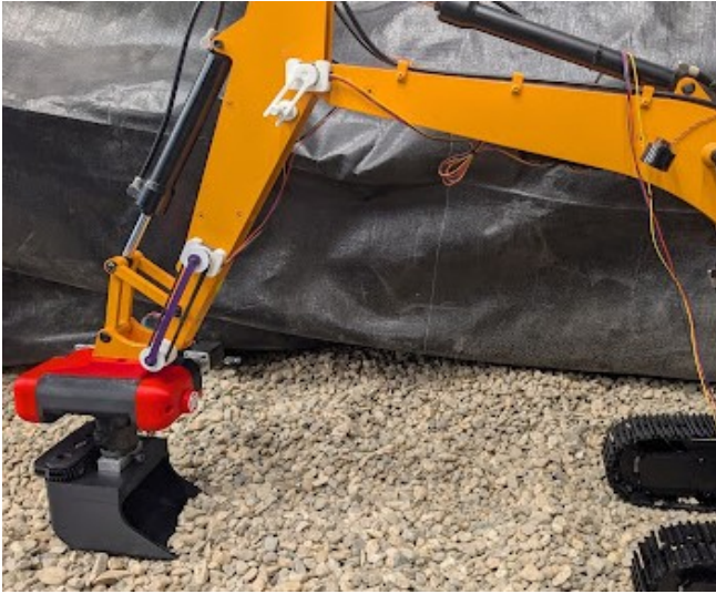
Figure 2: 1/12 Scale Earth Digger 4200XL Hydraulic Excavator used as the base research platform with installed tiltrotator.
