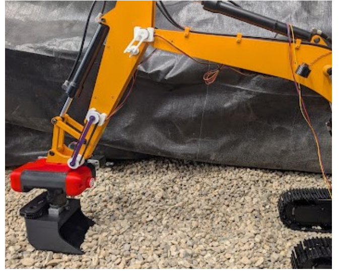
Figure 2: The finalized tiltrotator on the scale excavator
